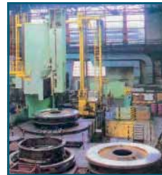
One of our machining center, having a maximum turning diameter of 12 m
