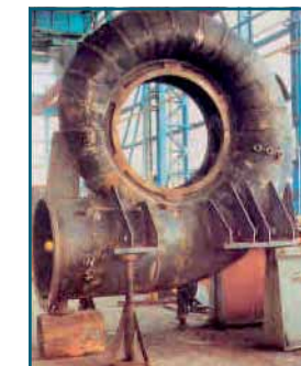
A low head Francis spiral case ready for machining, Karnah power station, Kashmir, India
